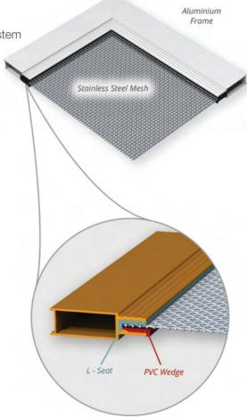
Defendoor TOUGH's patented security system includes a unique rib design which provides additional strength and resistance against intruders.
